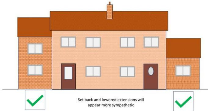
Extensions should be designed so that the main property is still the dominant building. The roof and eave lines should be lower than the existing house. Setting back the extension behind the front wall of the existing house can often help to achieve a satisfactory design.
